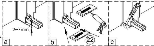
The setting wedge (No.22) will be needed if the profile is not level in 2-7mm.
