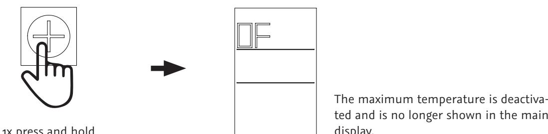
The maximum temperature is deactivated and is no longer shown in the main display.
