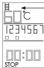
Flashes for selection of the temperature at 5°C increments.
