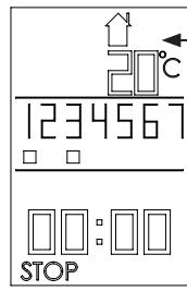
Flashes for selection of the temperature at 1°C increments.
